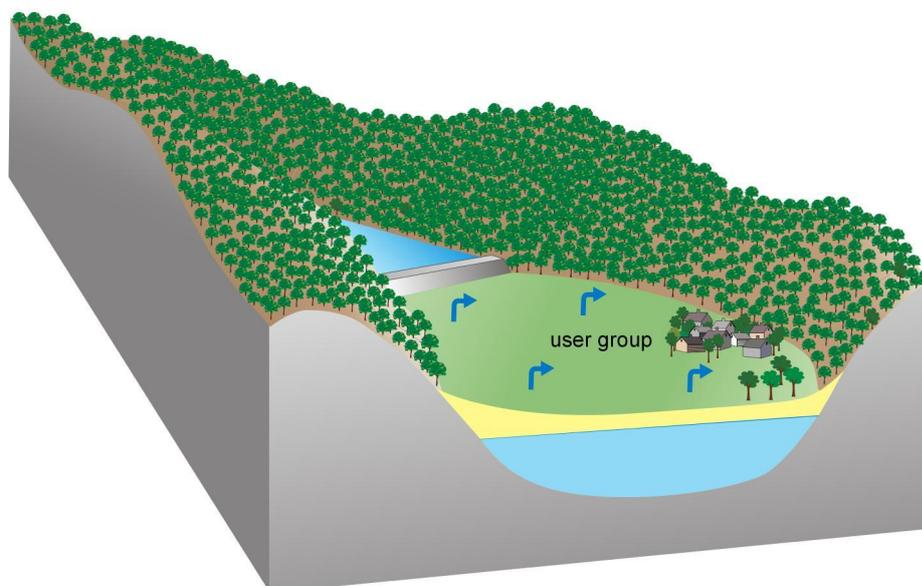
In the Arwari River Basin, the incised valleys in the upper reaches have natural boundaries to groundwater flow. They also form good sites for constructing high capacity check dams. Although groundwater is lost from the village catchment by lateral flow down-gradient, the influence of abstraction beyond the village boundary is not likely to be significant.
