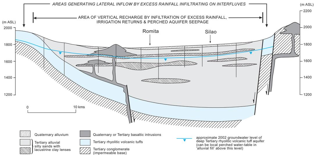
**Figure 2 : Schematic hydrogeological cross-section of the Silao-Romita aquifer system**
