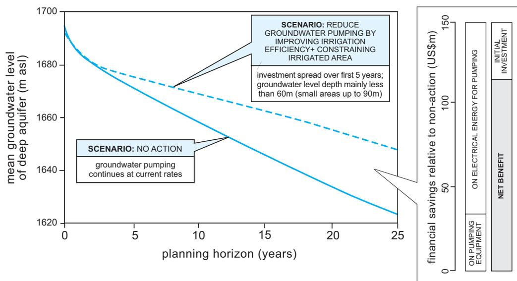
**Figure 4: Output of management scenario modelling for the Silao-Romita aquifer system using current MODFLOW numerical aquifer model integrated with economic data for selected agro-production regimes**
